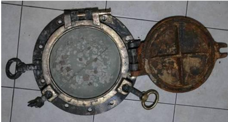
The cover (the Hatch) built from steel is corrosive in water.
